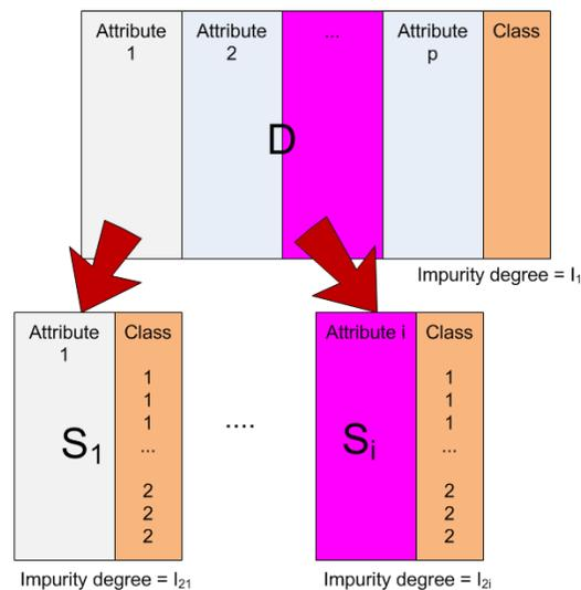
From table D and for each associated subset  $S_i$ , we compute degree of impurity. We have discussed about how to compute these indices in the previous section.
