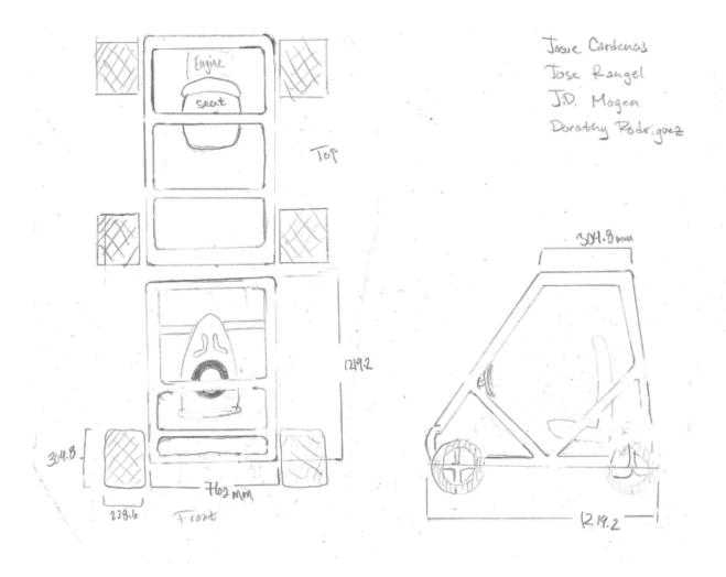
Figure: Sample dimensions of the proposed vehicle
