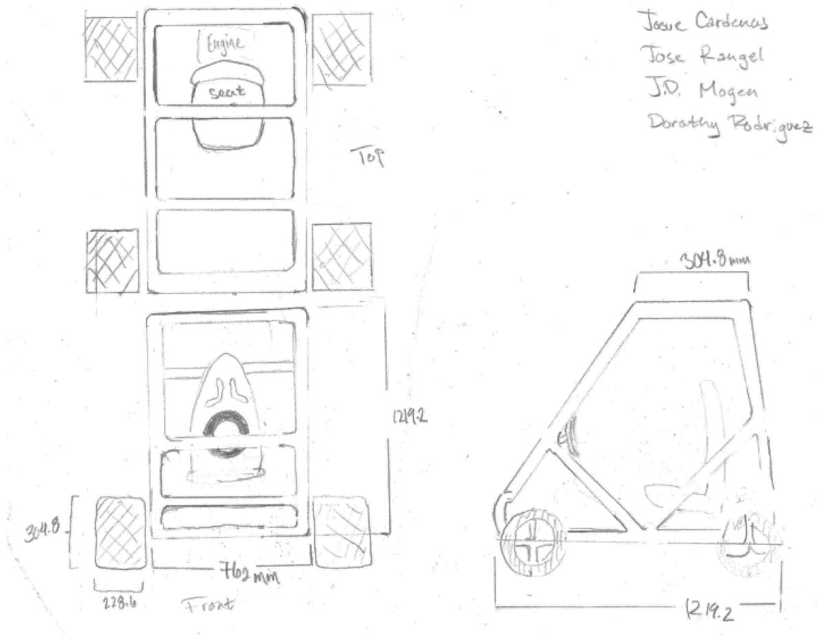
**Figure:** Sample dimensions of the proposed vehicle
