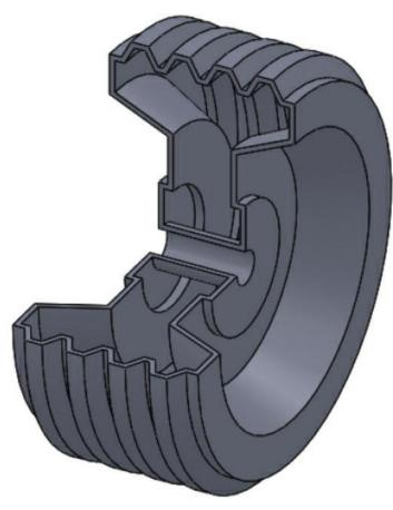
**Thin Feature** Angle of Rotation=270 degrees Thin thickness=5mm
